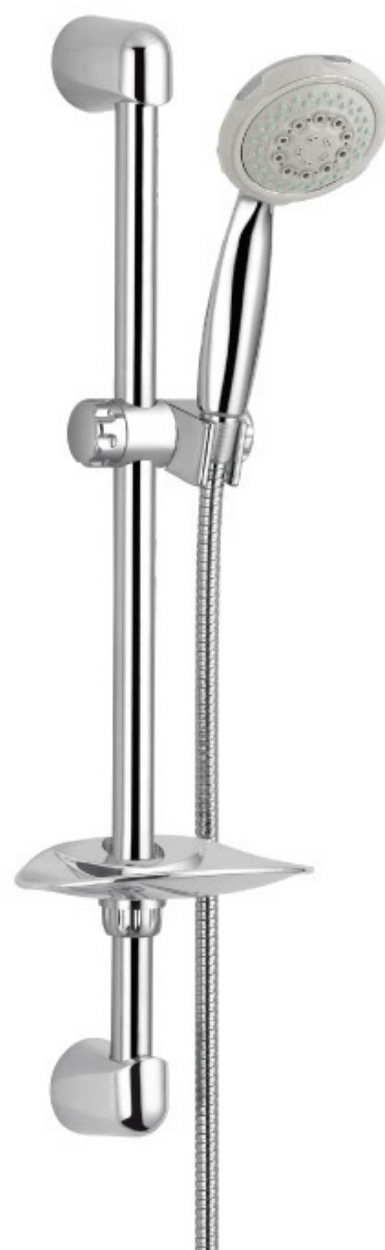
S6508WB+R1160B+H109 •Hand shower: S6508WB(5 functions, ø100mm,ABS) •Sliding bar: R1160B(ø25mm-L680mm,S/S) •Hose: H109(Double lock ,Flexible,1500mm,S/S)
