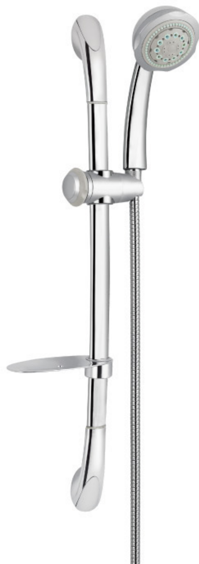
S5858WB+R1172B+H109 •Hand shower: S5858WB(5 functions, ø95mm,ABS) •Sliding bar: R1172B(30*15mm-L680mm,S/S) •Hose: H109(Double lock ,Flexible,1500mm,S/S)
